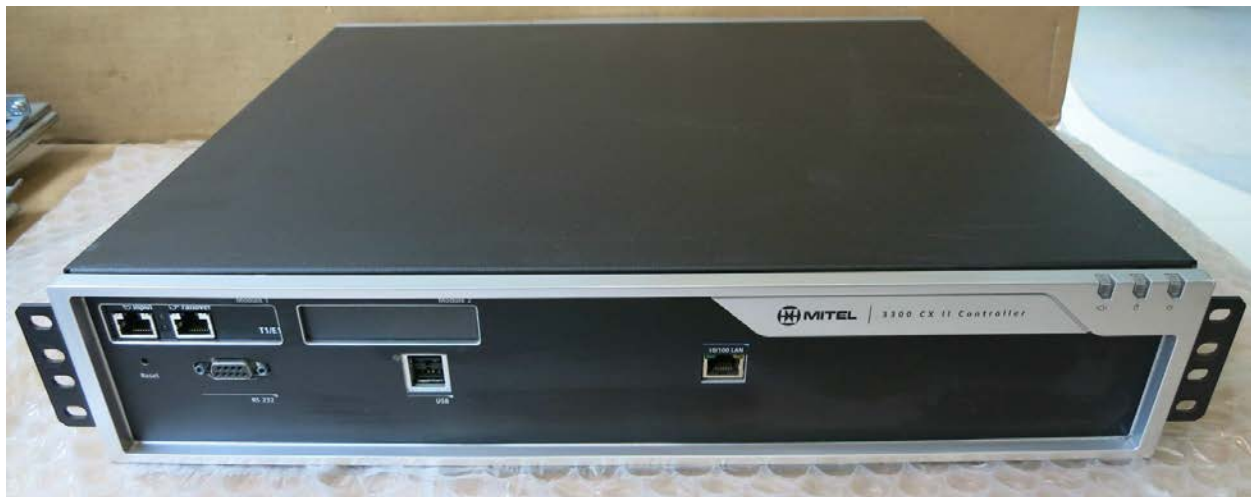
Figure 28. VoIP Hybrid Telephone System (only the server is illustrated)
